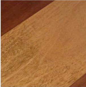
Grain discolouration – water based polyurethane
